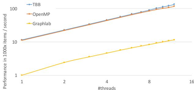
Fig. 3. Performance of the multi-core BPMF on the ChEMBL dataset in number of updates to  $U$  and  $V$  versus the number of parallel threads.
